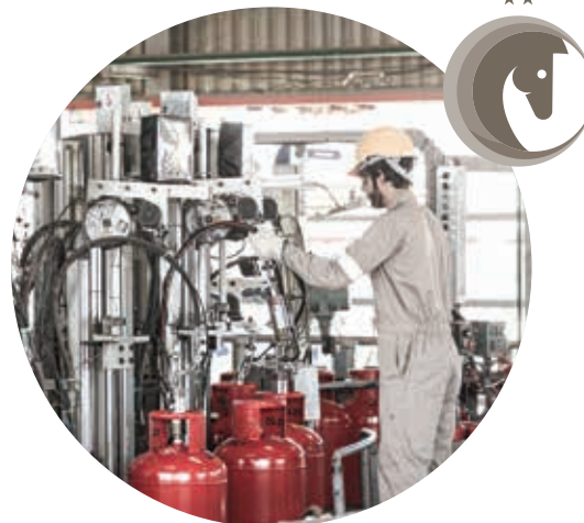
EMGAS Cylinder filling operation
